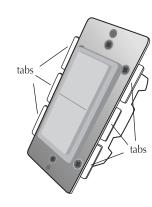
Step 4. When proper wiring is completed, secure the module to the wall box. Restore power to the circuit to test if the connected load or lighting can be turned ON/OFF, or Dimmed (when used with WD-100 dimmer only) manually by the rocker on the auxiliary switch(es) wired before remounting the wall plate.
